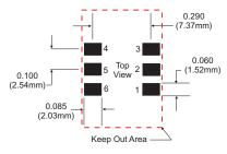
Keep Out Area Note: Do not route any traces under the device in the keep out area.
