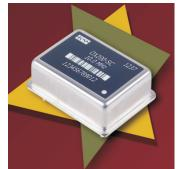
The OX-200-SC is a 10.0 MHz, 12 Vdc, ovenized third overtone SC Cut crystal oscillator with Electronic Frequency Control (EFC) in a CO-8 package. Its frequency stability is ±1.5 ppb within the temperature range of 0° to °70C. Frequency calibration is guaranteed to be less than ±25 ppb with
