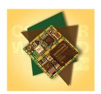
The TI125 has an on-board programmable NCO oscillator that outputs a synthesized frequency up to 30 MHz that is steered by the GPS receiver. The self-survey mode of operation allows the receiver to enter a position hold mode to allow accurate timing to be continued with only one satellite being tracked.
